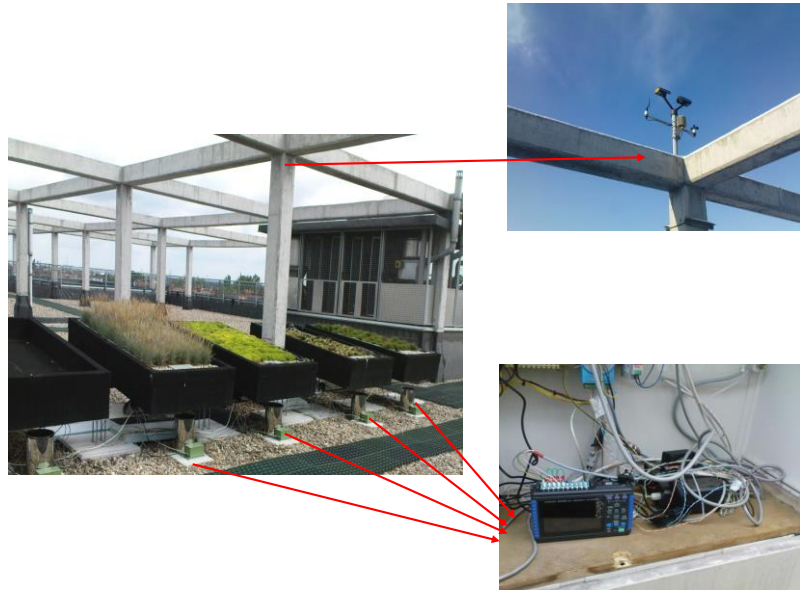
Fig. 1 Green roof models on the roof of the Science and Education Center, Wrocław University of Environmental and Life Sciences, with the precipitation measuring system (distrometer - laser precipitation sensor) and runoff measuring system (electronic devices placed under the roof platforms to continuously measure the amount of runoff from test plots, connected to Memory Hilogger 8430-20 by HIOKI)
