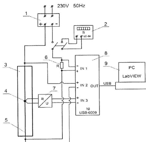
Fig. 1. Experimental set up to measure thermal conductivity of liquids:
