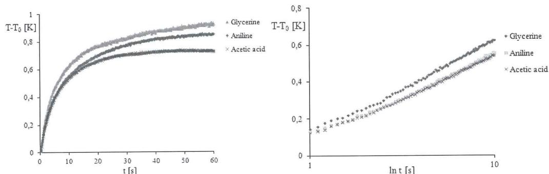
Fig. 2. Temperature of heating wire as a function of time in three tested samples of liquid:
