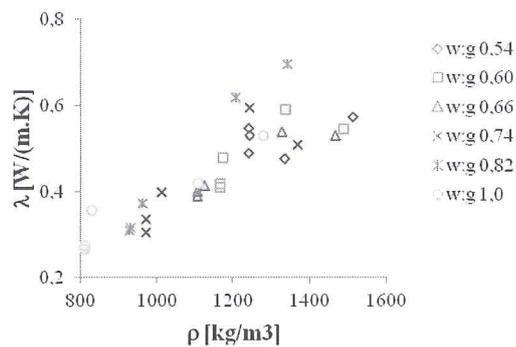
Fig. 5. Graphs of dependencies  $\lambda = f(\rho)$  of samples with admixture of polymer for different ratios of water to gypsum
