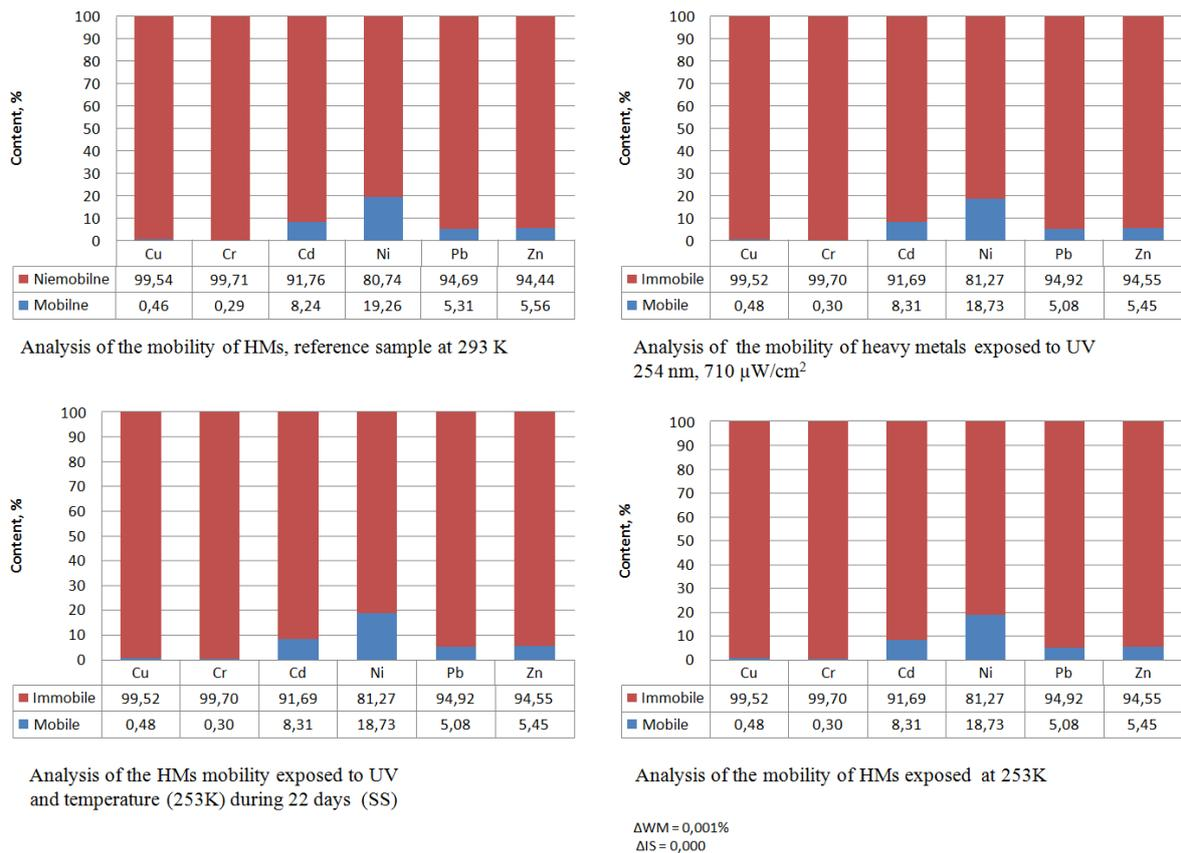
**Fig. 7.** Effect of sewage sludge weathering on heavy metal mobility
