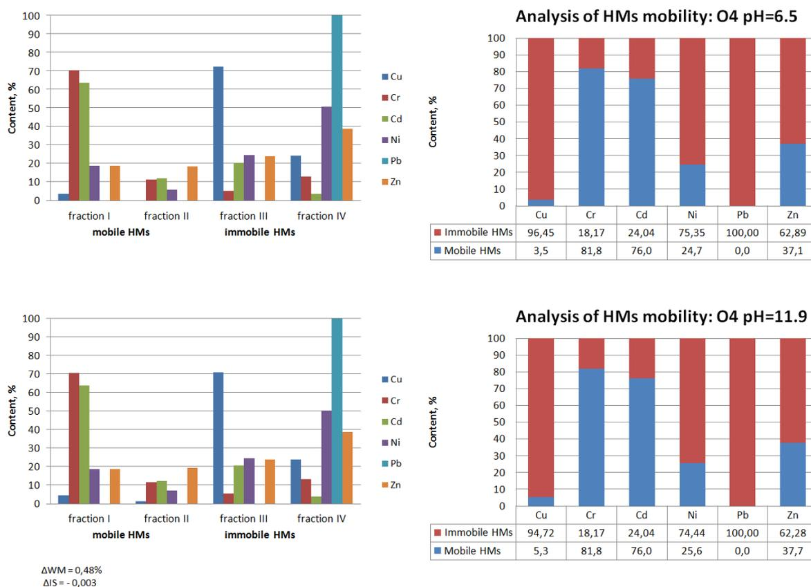
**Fig. 6.** Effect of sewage sludge alkalisation on heavy metal mobility (pH=11.9)
