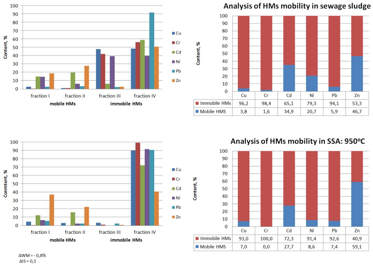
**Fig. 9.** Effect of sewage sludge incineration on heavy metal mobility
