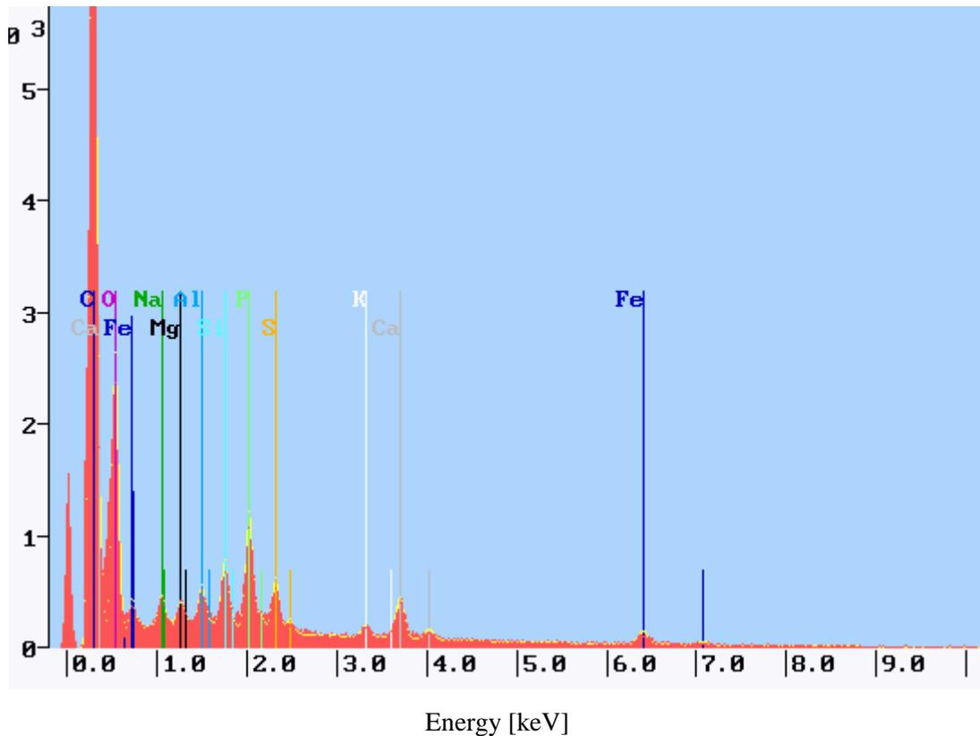
**Fig. 2.** X-Ray microanalyses spectrum of the sewage sludge sample from the sewage treatment plant in Daleszyce
