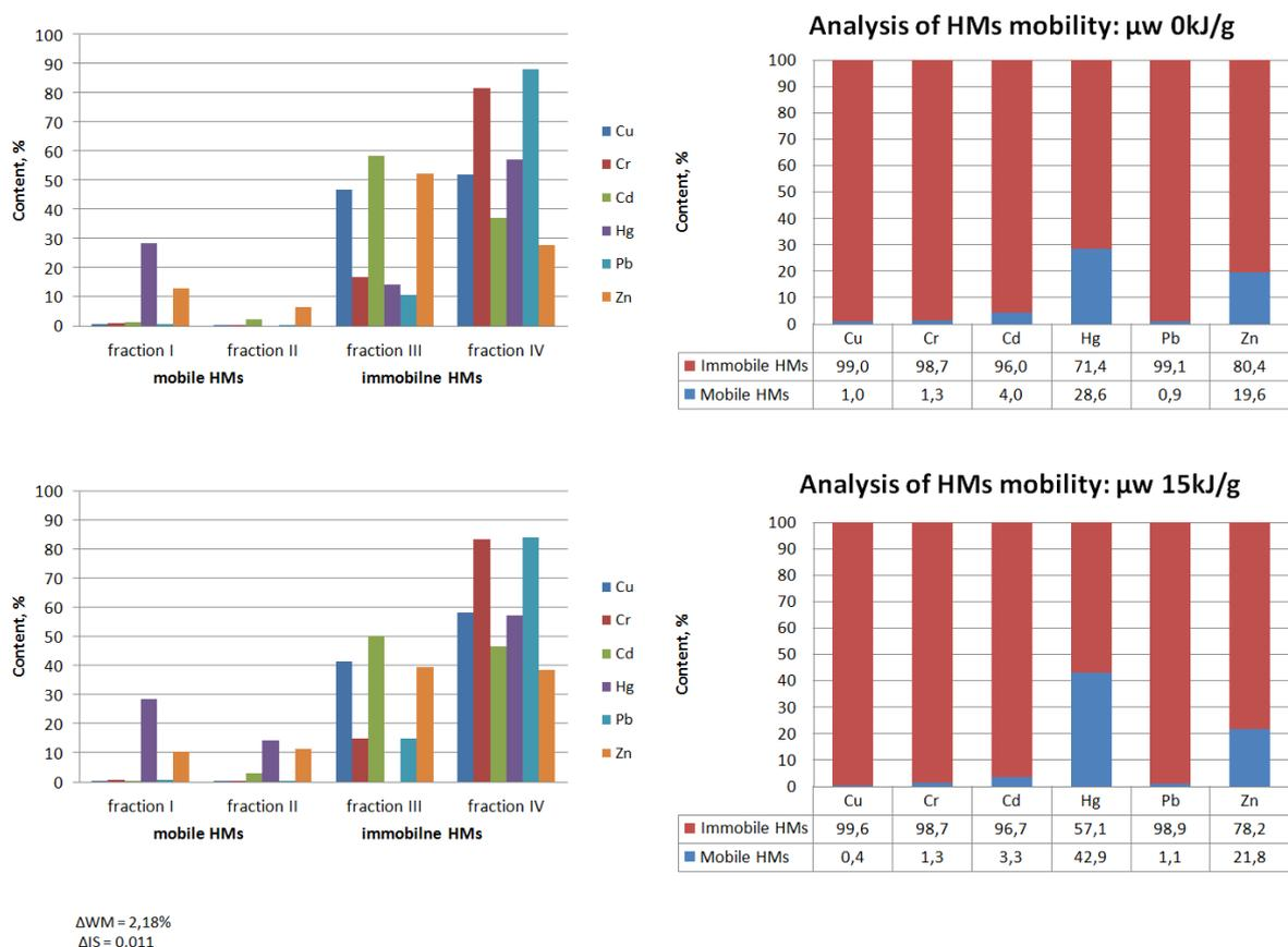
**Fig. 1.** The effect of microwave radiation (2450 MHz) on heavy metal mobility in sewage sludge collected from the sewage treatment plant in Sitkówka-Nowiny
