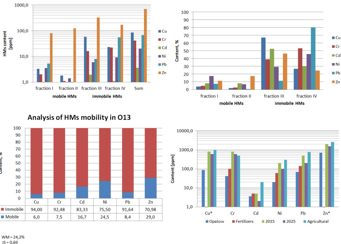
**Fig.5.** Mobility of heavy metals in the sewage sludge on the example of the sewage treatment plant O13 and the metal content in accordance with the legislation in force and planned alterations [3,6,16]
