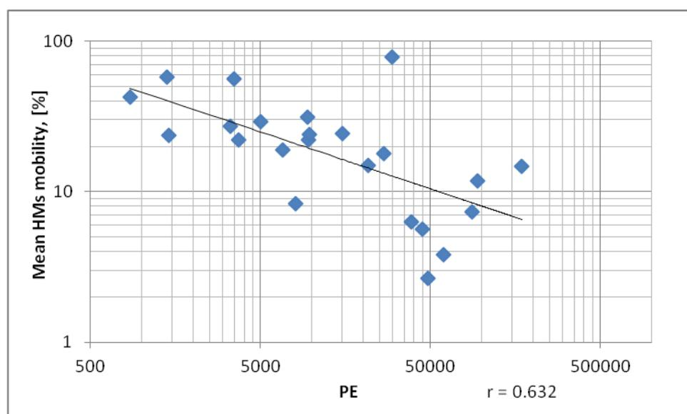
**Fig. 3.** The correlation between the mean heavy metal mobility and the sewage treatment plant capacity O1–O23
