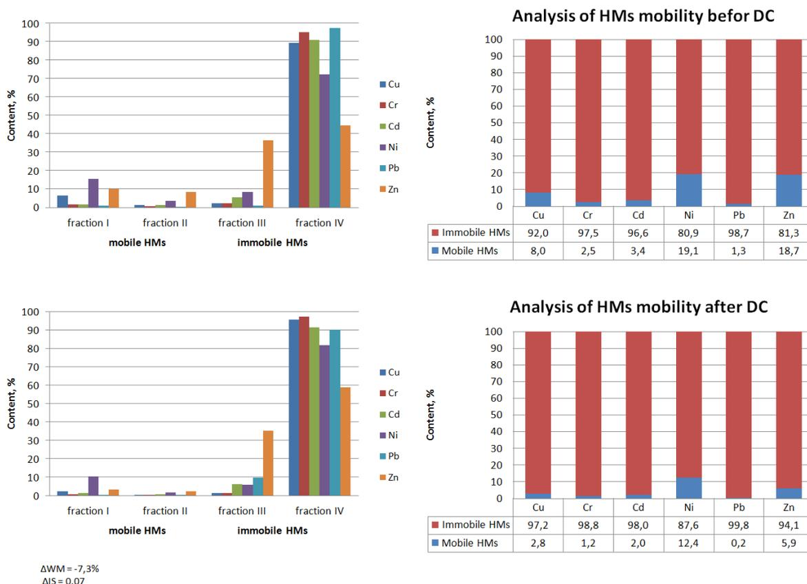
**Fig. 8.** Effect of mesophilic digestion of sewage sludge on heavy metal mobility
