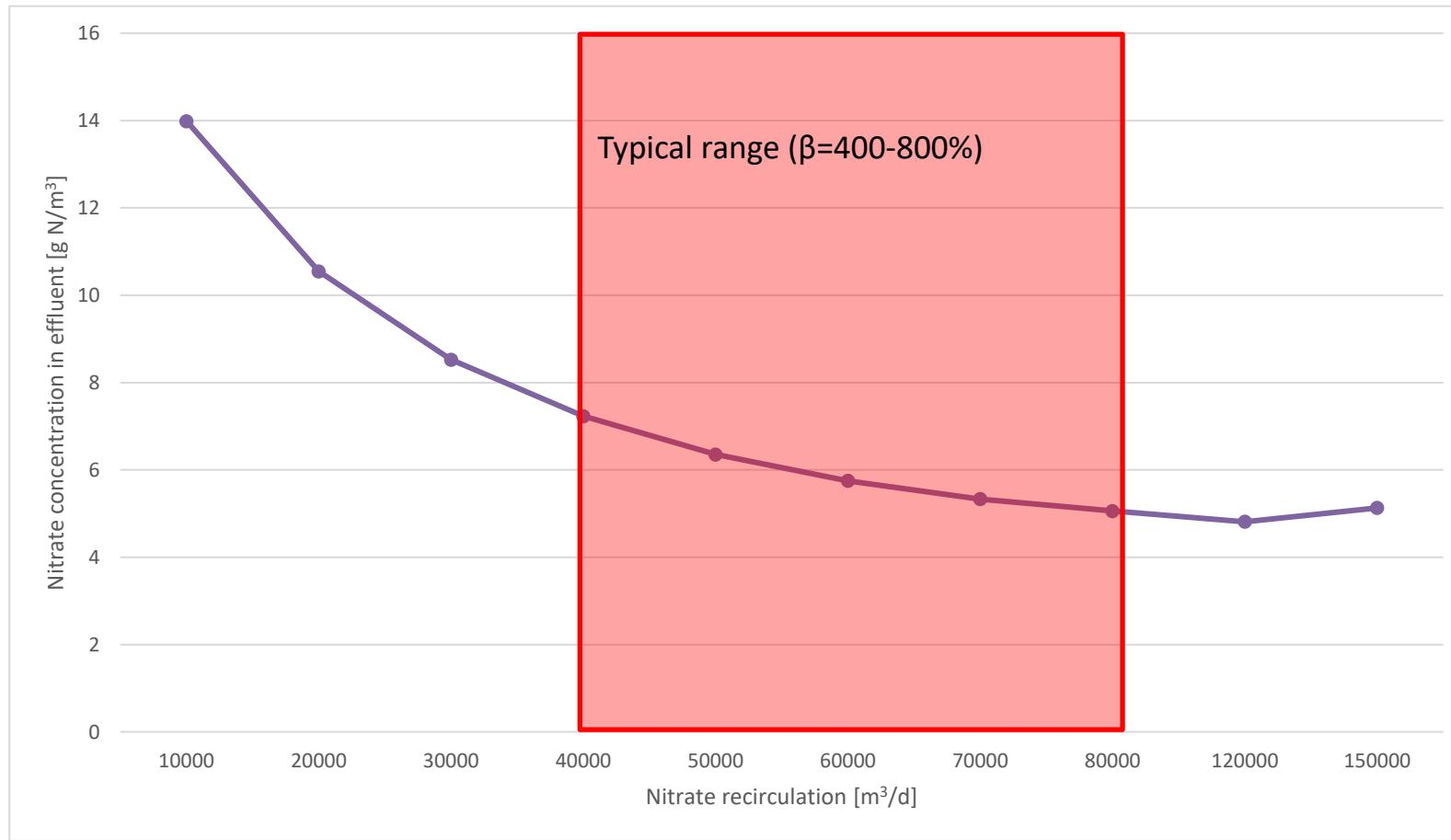
Wastewater flow = 10 000  $\text{m}^3/\text{d}$
