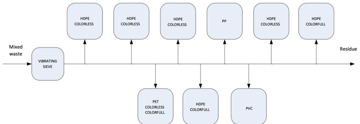
Rysunek 1. Schematic of plastic separation during manual sorting [1]
