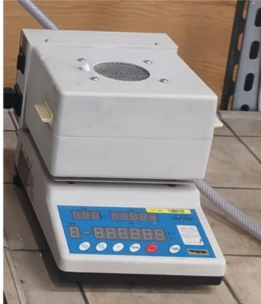
Figure 6. Moisture analyzer
