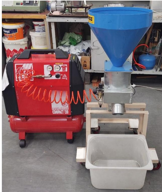
Figure 3. Metal separator for ferrous metals
