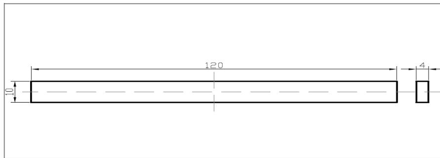
Figure 3. Dimensions of impact test samples
