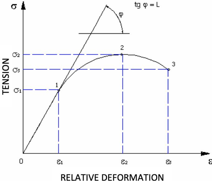
Figure 4. Schematic diagram of the stretching of plastic mixtures
