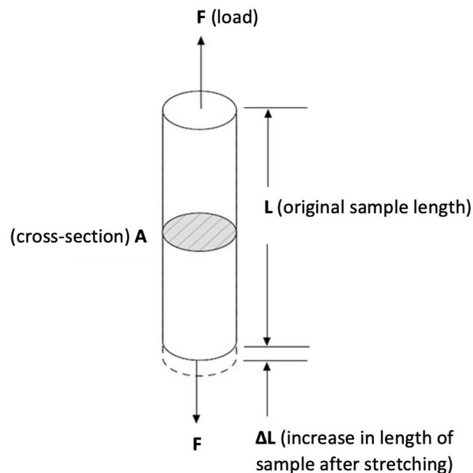
Figure 1. Schematic diagram of the distribution of forces and deformations in the sample [1]
