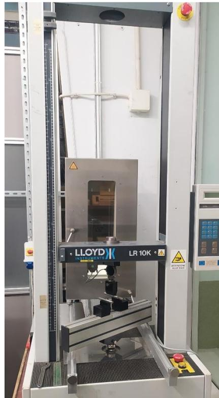
Figure 3. LLOYD LR 10K testing machine with LLOYD TC540 thermal chamber
