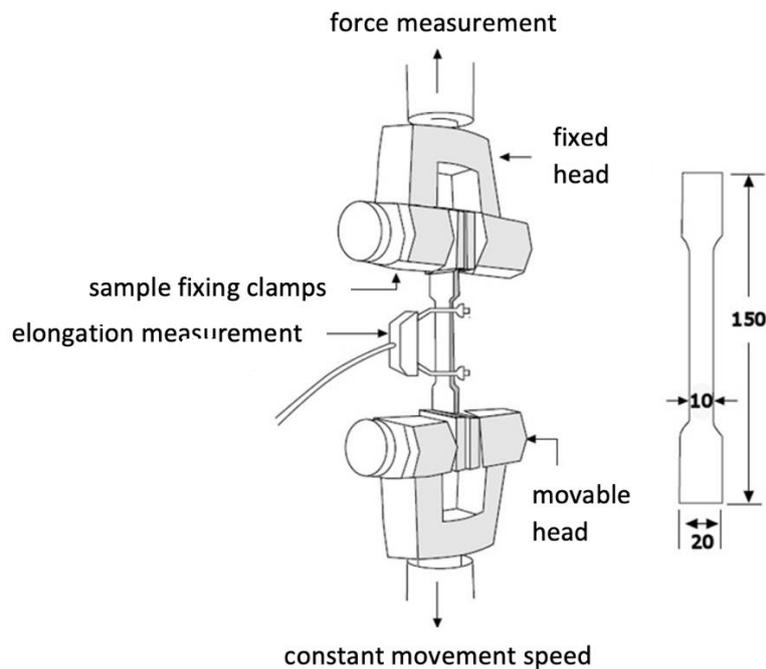
Figure 2. Schematic process of sample stretching [1]
