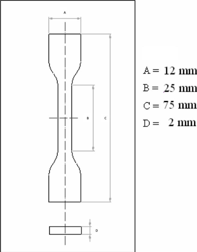
Figure 5. Dimensions of samples for strength tests
