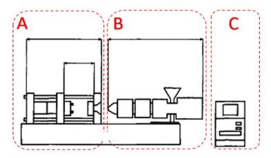
Figure 6. Functional components of an injection molding machine [2] A - Tooling system, B - Plasticizing system, C - Drive and control system
