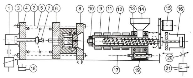
Figure 5. Schematic of a screw injection molding machine with basic components: 1 – drive cylinder for the table, 2 – guiding columns for the table, 3 – height adjustment nuts for the mold, 4 – rear fixed table, 5 – toggle lever system, 6 – moving table, 7 – injection machine buffer, 8 – front fixed table, 9 – injection cylinder, 10 – injection nozzle, 11 – screw, 12 – heaters, 13 – cooling system for the cylinder's feed zone,
