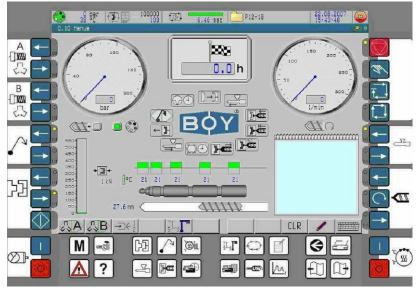
Figure 7. Control panel of the BOY 35A screw injection molding machine
