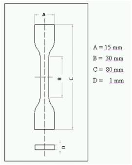
Figure 3. Dimensions of tensile test samples in accordance with ASTM D 0638.
