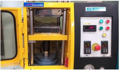
Figure 1. Hydraulic press with heating and cooling plates (LabTech LP20-B).
