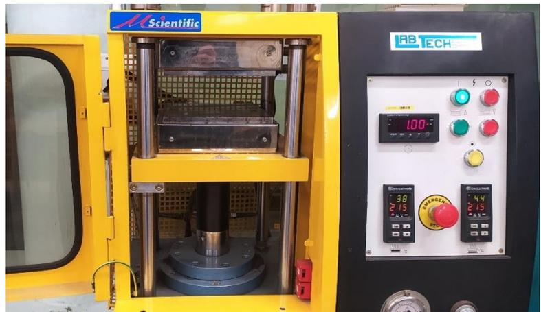
Figure 1. Hydraulic press with heating and cooling plates (LabTech LP20-B).
