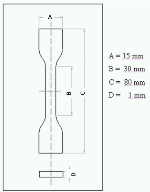
Figure 3. Dimensions of tensile test samples in accordance with ASTM D 0638.
