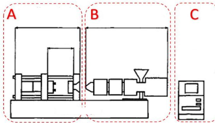
Figure 6. Functional components of an injection molding machine [2]
