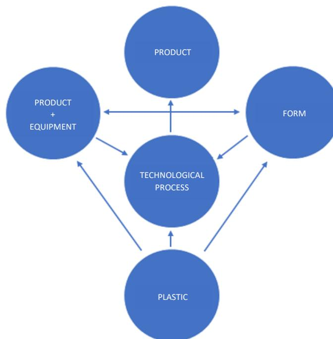
Figure 4. Factors affecting part quality and production efficiency [2].
