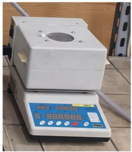
Figure 6. Moisture analyzer
