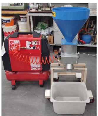
Figure 3. Metal separator for ferrous metals
